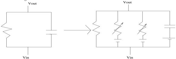
Now, we have a cable with variable conductances. The problem is to find the new cable equation. This can be done, but we will only get to the variation of voltatage with respect to time.
